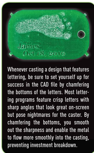
Whenever casting a design that features lettering, be sure to set yourself up for success in the CAD file by chamfering the bottoms of the letters. Most lettering programs feature crisp letters with sharp angles that look great on-screen but pose nightmares for the caster. By chamfering the bottoms, you smooth out the sharpness and enable the metal to flow more smoothly into the casting, preventing investment breakdown.
