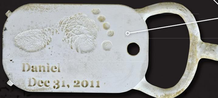
After milling a second wax and changing the position of the sprues, RW's team succeeded in achieving the desired detail. "We placed the sprues as far away from the lettering as possible and angled them," says Melissa Holthoff. "They go up around the piece and then into the lettering, giving the molten metal time to slow down before it meets the details."
