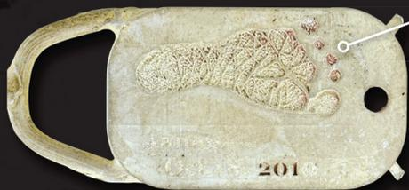
The first attempt at casting, with 3 mm sprues placed at both sides of the pendant's base fed by a larger 4 mm sprue, failed.
